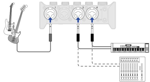
2. Set MIC O GUITAR and according to the connected device.
