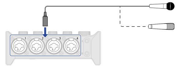
**2.** When connecting a mic to the Input 1 jack, set  $\frac{\text{MIC}}{\text{LINE}} \bigcirc \frac{\text{GUITAR}}{\text{GUITAR}}$  to MIC/LINE.
