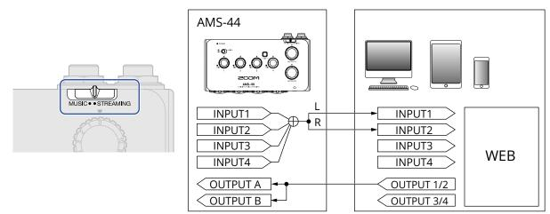
When the AMS-44 Stereo Link switch is on, Input 3 (left) and Input 4 (right) function as a stereo input. ( $\rightarrow$  Stereo link overview)
