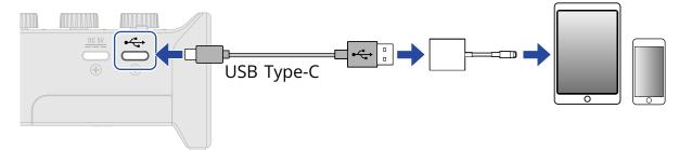
To connect smartphones and tablets, prepare USB cables and adapters that match their connectors as necessary.
